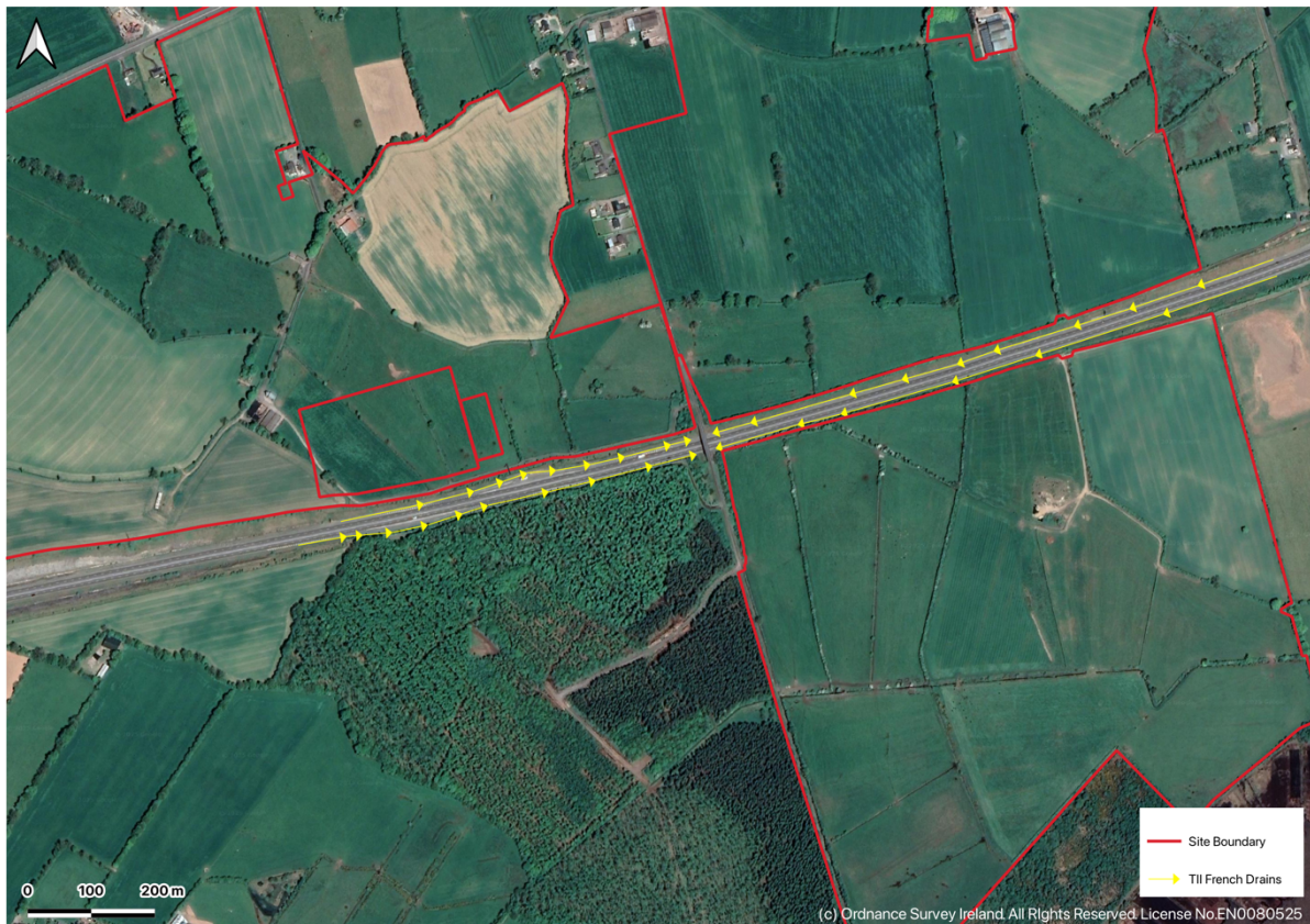
Figure 9 – French drains and their flow direction along the M6 towards Kil1
