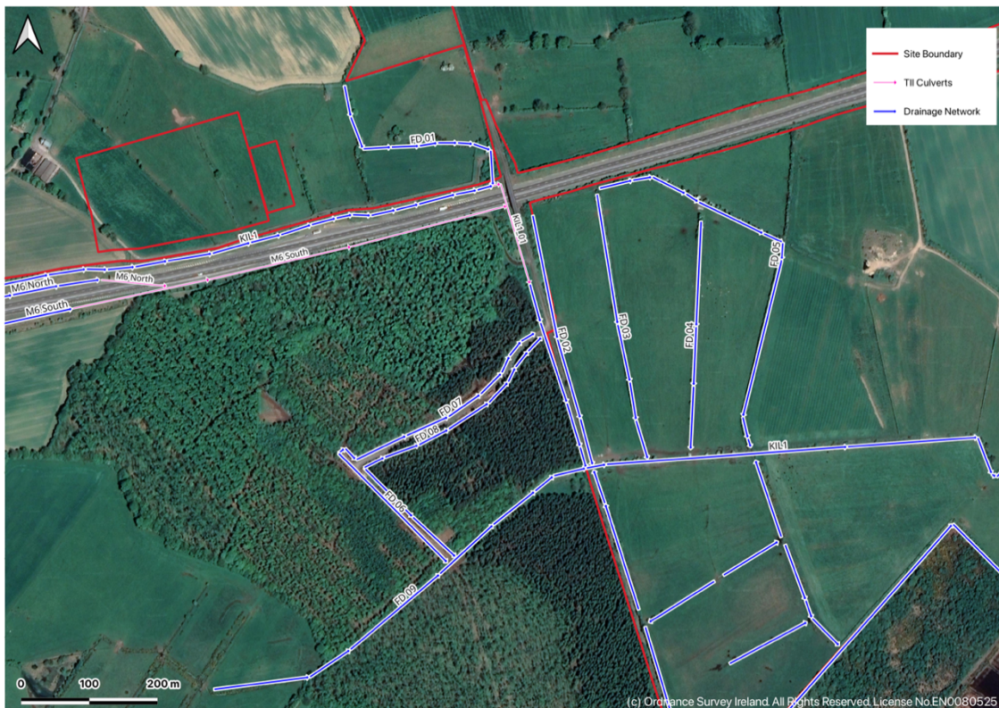
Figure 8 – Kil1 detailed drainage network
